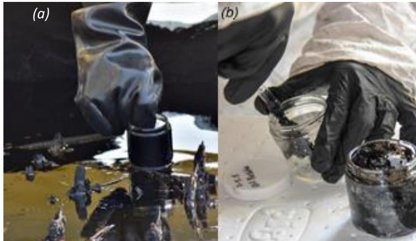
Figure 10. Post-burn residue sample collection (a) and preparation (b) for chemical analysis.
