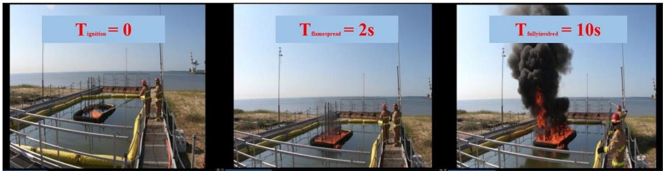
Figure 45. Ignition, flame spread and fully involved times for large-scale crude ISB.
