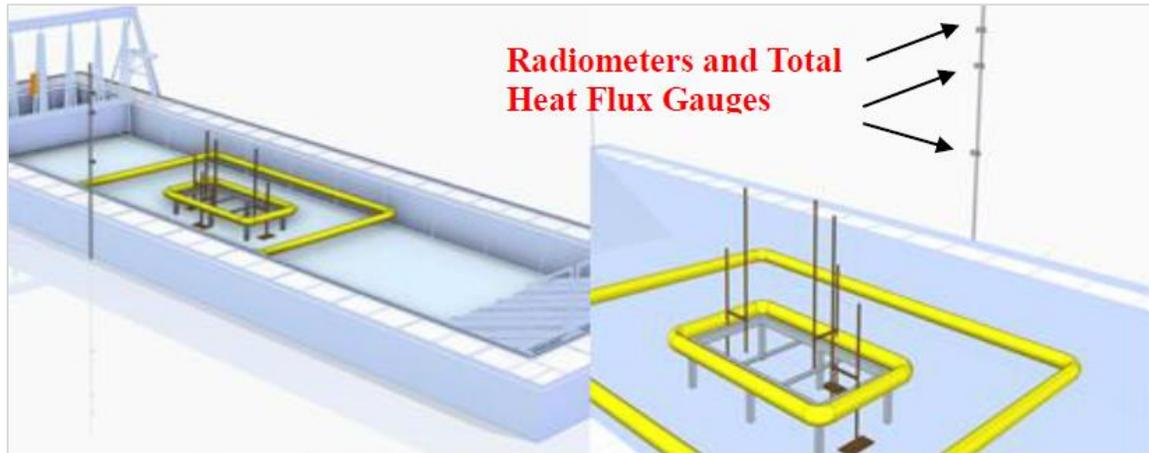
Figure 38. Large-scale ISB heat flux gauge setup.
