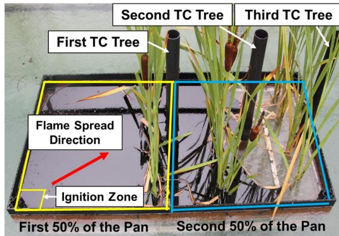
Figure D-2. Picture of the zones used to calculate the flame spread rates in Table D-2.
