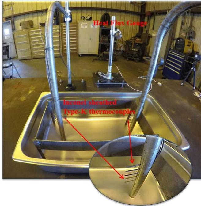
Figure 6. Small-scale instrumentation layout of thermocouples and heat flux gauges.
