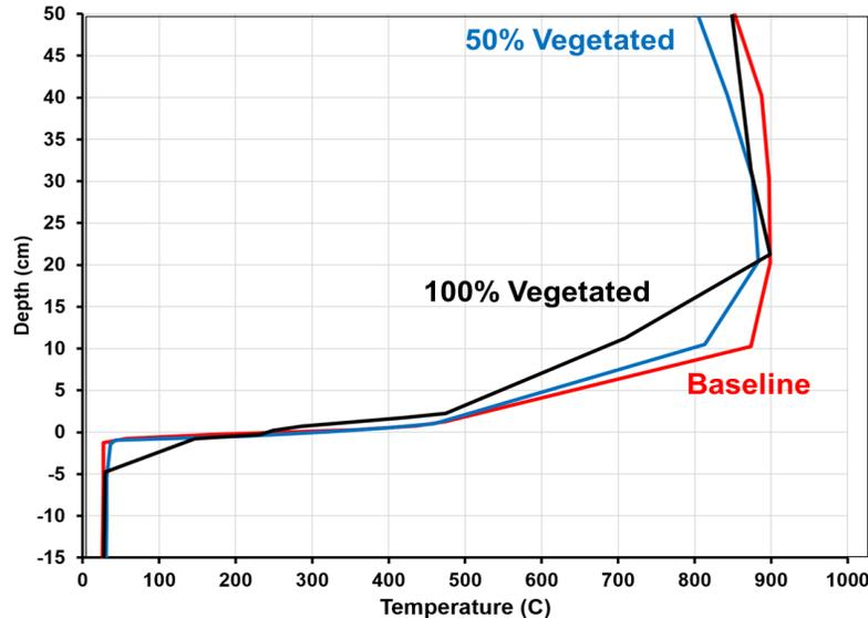
Figure D-6. Temperature profiles at the pan center after 1 minute reaching to the  $t_{100}$ .
