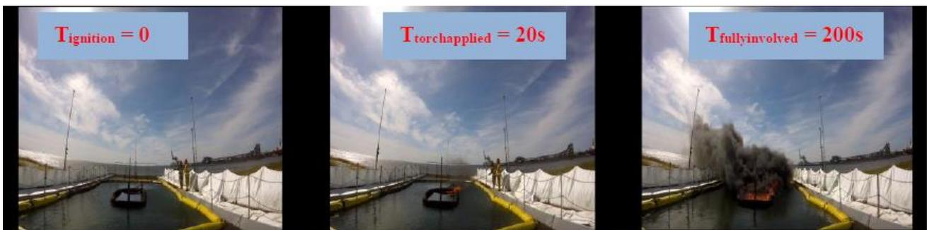
Figure 46. Ignition, flame spread and fully involved times for large-scale RMG 380 ISB.
