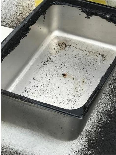
Figure 12. Hardened residue around pan lip and small tar balls immediately following small-scale ISB.
