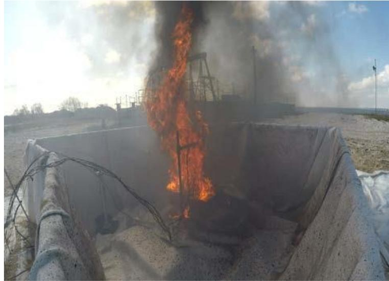
Figure 14. Violent fire growth and swirling behavior observed during small-scale test (S3).
