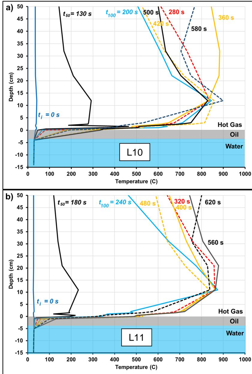
Figure D-7. Temperature profiles of the mesoscale experiments with double oil mass.
