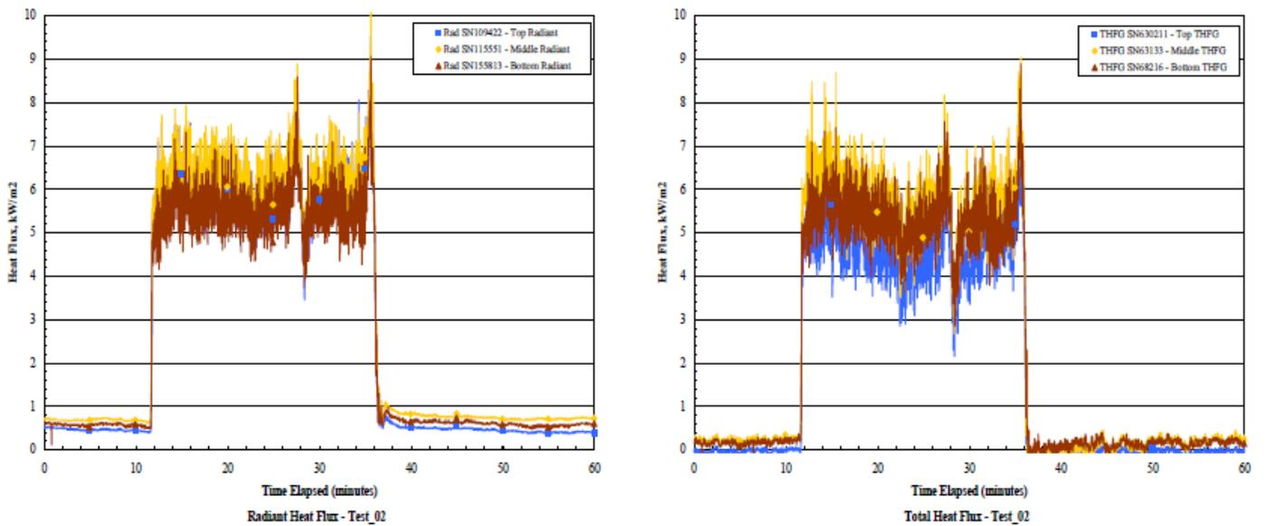
Figure F-8. Large-scale test L2 (crude oil with vegetation), radiant and total heat flux measurements.
