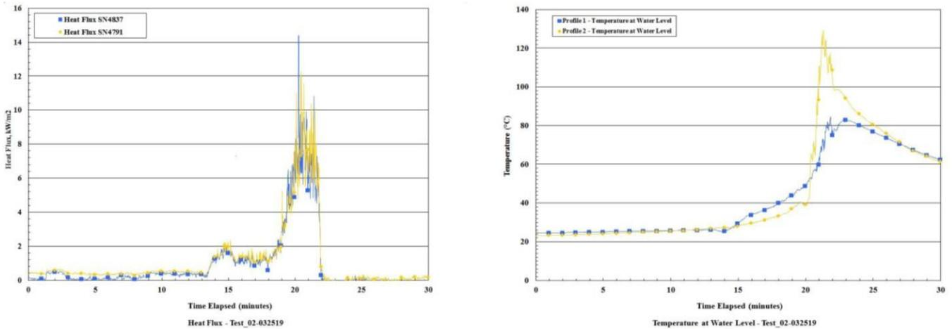
Figure C-2. Test 2 total heat flux measurement and temperature at the water level.
