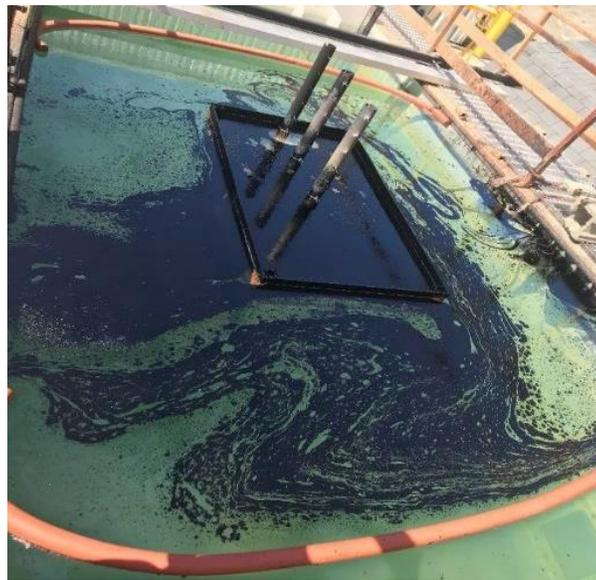
Figure 32. Splatter outside of the burn area from boil over during mesoscale ISB.
