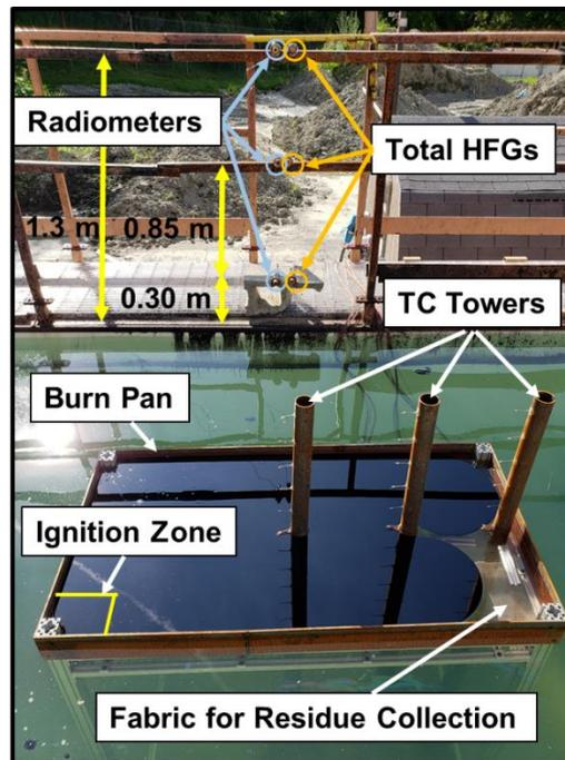
Figure 24. Instrumentation used in mesoscale experiments.
