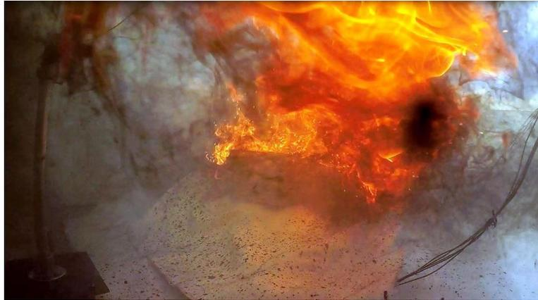
Figure 17. Boil-over and resultant splatter during small-scale ISB.
