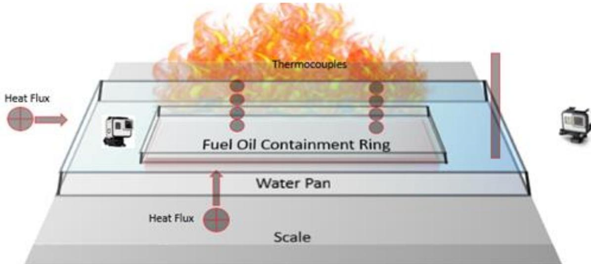
Figure 5. Sketch of small-scale pretest set-up showing scale, thermocouple, and heat flux instrument placement.
