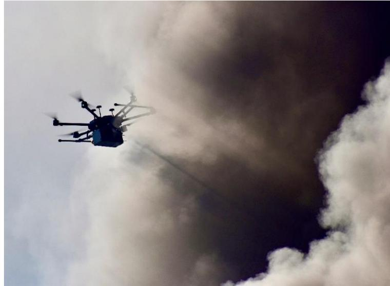
Figure 44. sUAS mounted air monitoring sensor package sampling inside the smoke plume.
