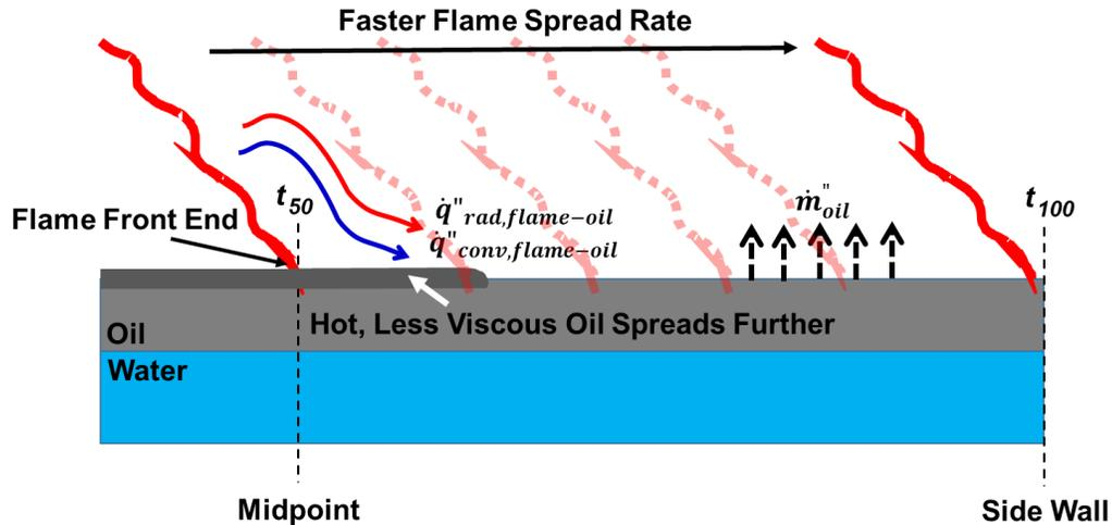
Figure D-3. Sketch of the faster flame spread in the second half of the burn pan.
