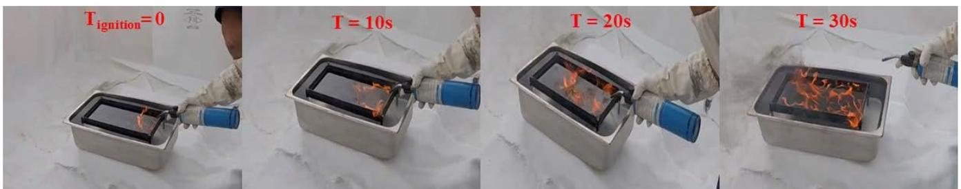
Figure 11. Propane torch ignition stages over time (T) of RMG 380, 10 mm thickness with no diesel accelerant.
