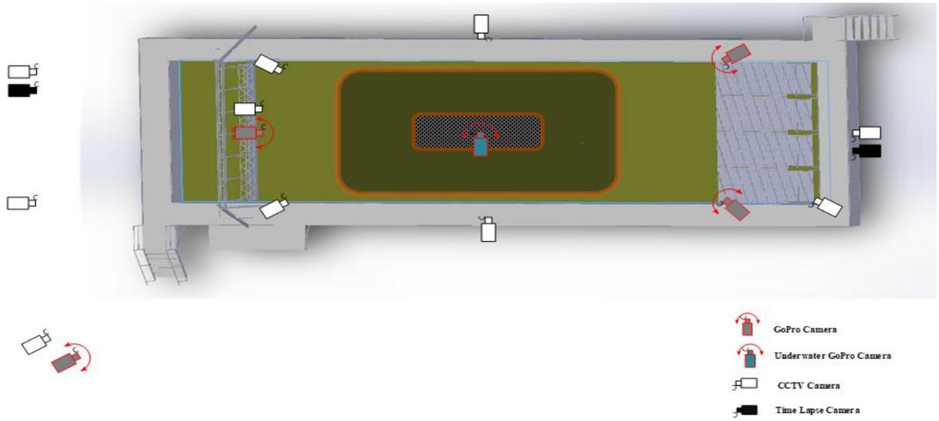
Figure 41. Stationary video placements for large-scale ISB tests.
