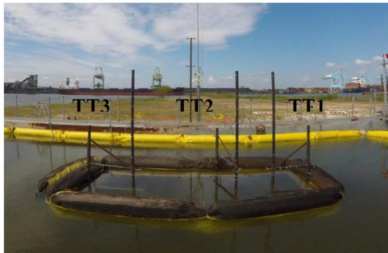
Figure 37. Placement of thermocouple trees during large-scale ISB tests.
