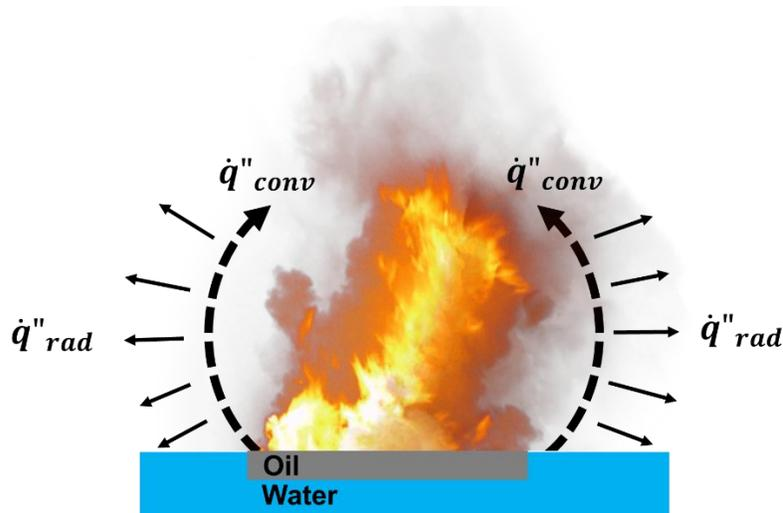
Figure D-9. Heat transfer mechanism from flame to ambient in an ISB.
