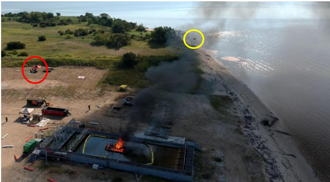
Figure 43. sUAS mounted with EPA sensor package (yellow circle) flying in ISB smoke plume.
