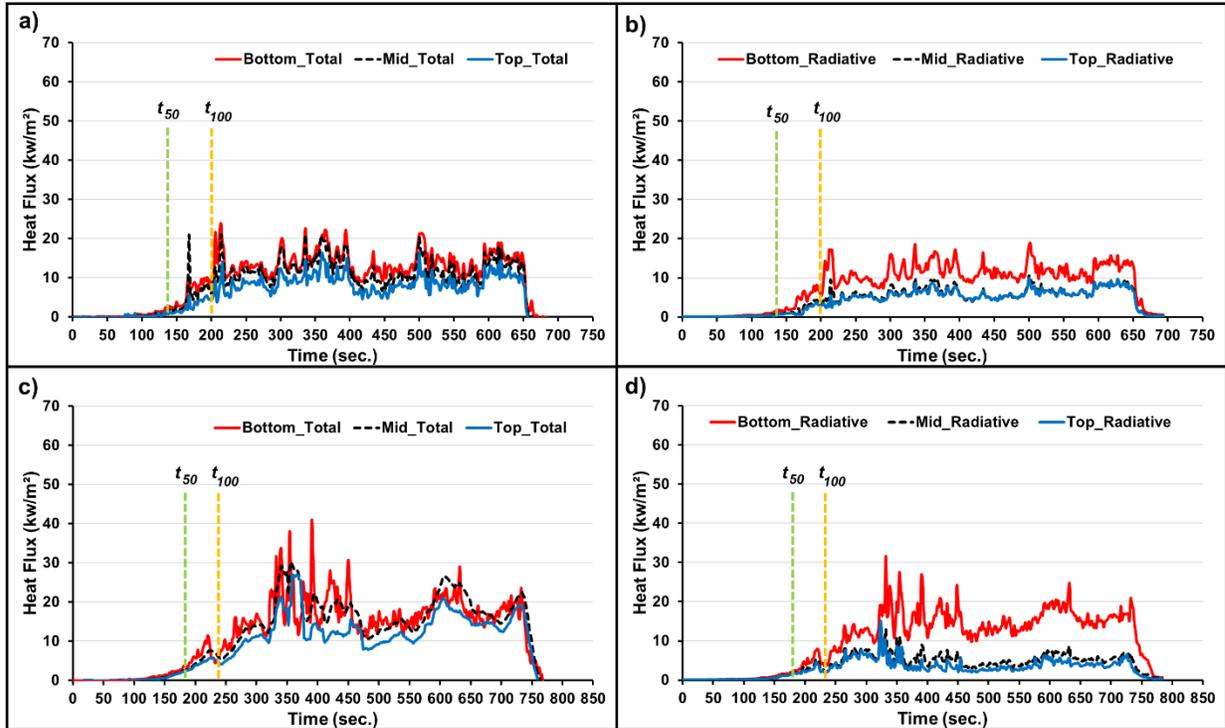
Figure D-10. Heat flux measurements of the mesoscale experiments with double oil mass.
