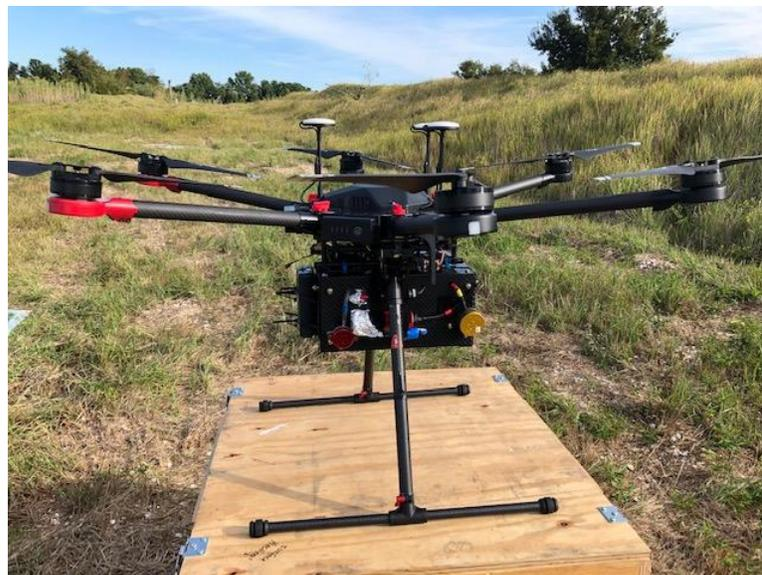
Figure 39. RDC's sUAS with EPA's Kolibri sampling system.
