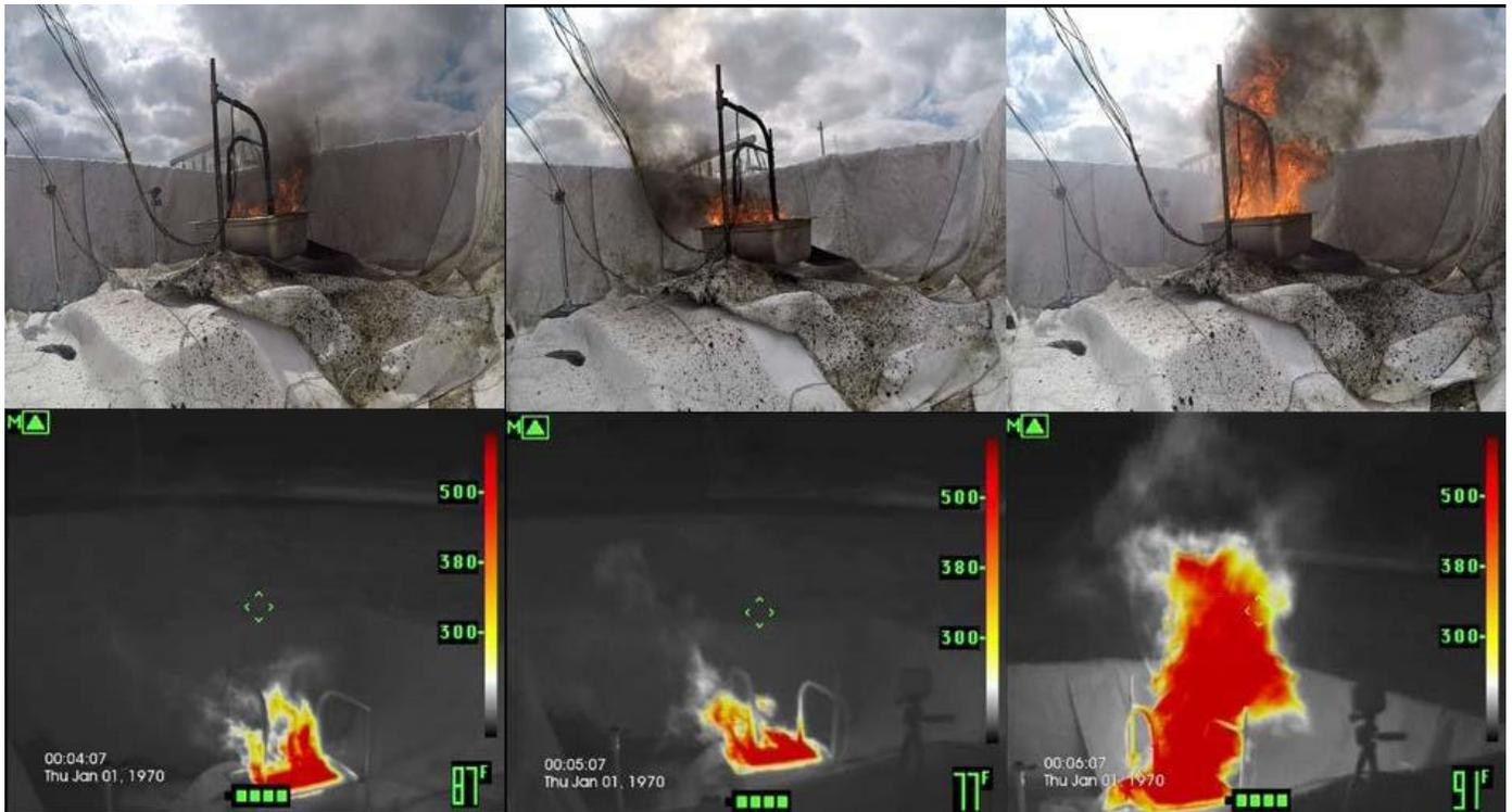
Figure 8. Visual screenshots and associated infrared images of fire spreading.
