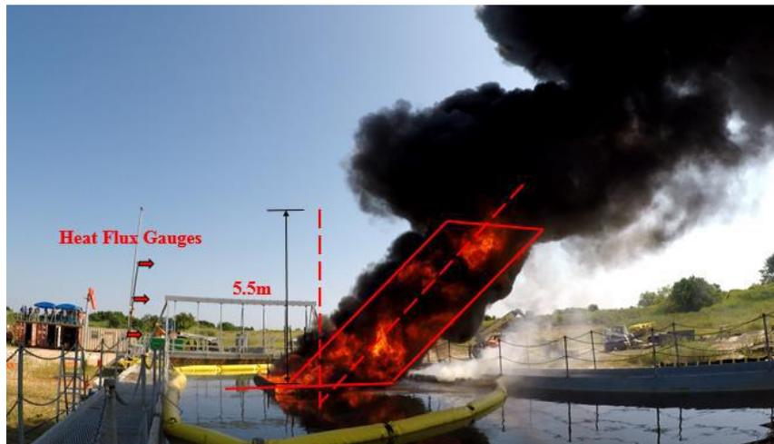
Figure 47. Large-scale flame and plume trajectory affected by wind (L1).
