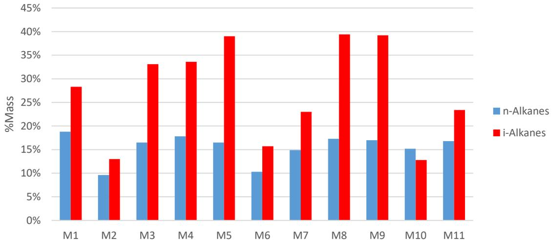
Figure 30. Total n- and i-alkane mass percentages in residue from mesoscale ISB of Bunker C Oil.
