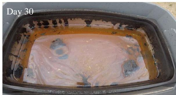
Figure 21. Oil residue and tar balls after thirty days of weathering.
