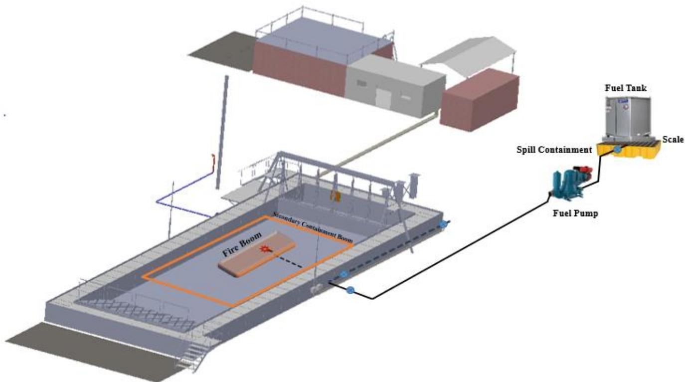
Figure 34. Flowing fuel system large-scale ISB.
